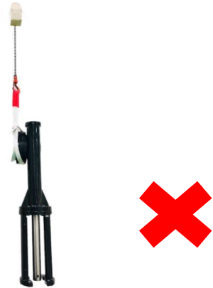
Error: Suspend the gearbox separately.
