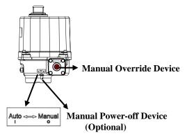
c. After finishing the manual override device operation, switch the actuator from manual operation (Manual) back to electrical operation (Auto).
