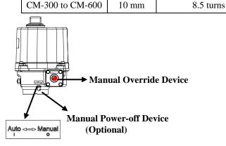
c. After finishing the manual override device operation, switch the actuator from manual operation (Manual) back to electrical operation (Auto).
