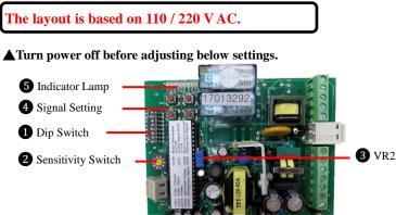
**1** Dip Switch Setting (Original Factory Setting : 1, 4, 8 ON)
