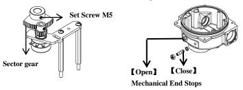
d. Refer to below illustrations to adjust the TC1 - TC4 to set the fully-open and fully-closed position.
