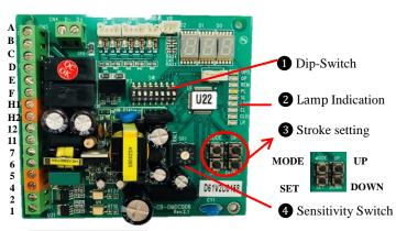
1 Dip-Switch Setting (Original Factory Setting: 1, 4, 8 ON)
