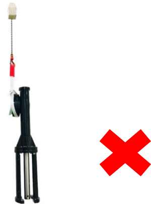
Error: Suspend the gearbox separately.
