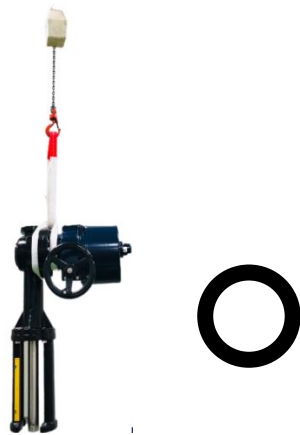
Correct: The actuator is suspended with the gearbox.
