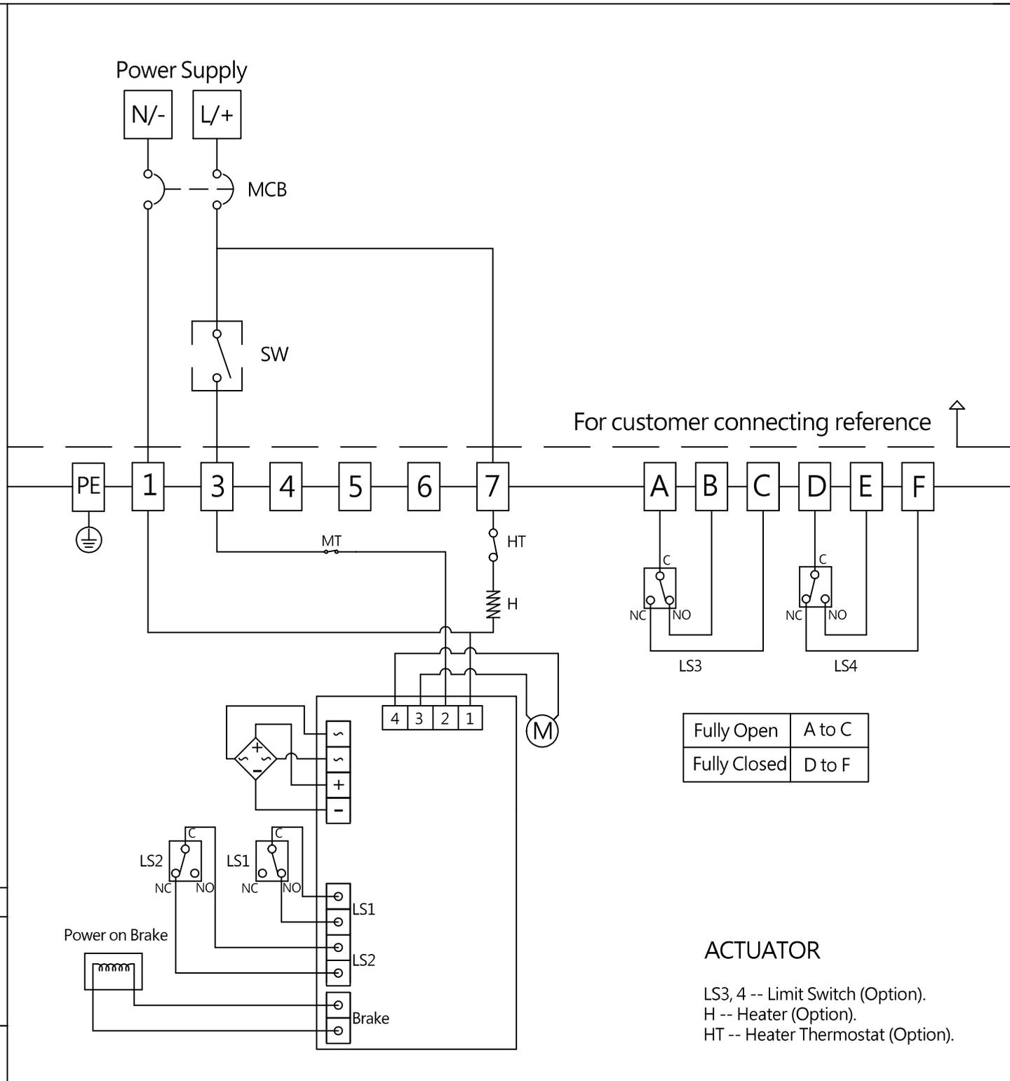
Wiring Diagram NO: 02-008-02-04-01-32-2-041
